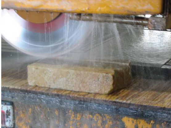
Figure 1: Regeneration of disc in abrasive material
